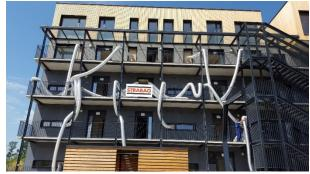
Figure 8. Air tightness measurements of the building envelope.
