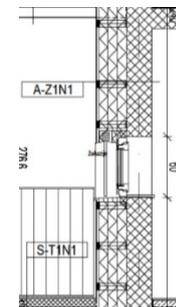
**Figure 4.** Cross section of reinforced concrete bearing wall.
